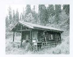
On the earliest nineteenth-century houses, the roof was made of split logs or rough wood planks that ran from the roof peak to the eaves. These rough roofing boards were later covered with split shingles to make the roof more weather tight. At the turn of the twentieth century, metal roofs were favored when the material was made available with the advent of railroads.
